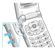
In Idle Mode with the folder open, you can also adjust the keypad tone volume using these keys.
