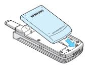
5. Press the battery down until it clicks into place. Make sure that the battery is properly installed before switching the phone on.
