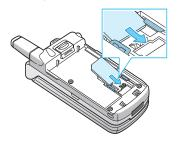
**Note**: When you need to remove the SIM card, slide it, as shown, and take it out of the socket.
