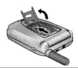
3 Insert the SIM card into the SIM card door with the notch in the upper left corner and the gold plate facing down.
