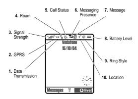
1. Data Transmission Indicator – Shows connection and data transmission status. The Bluetooth® wireless connection indicator ≯ shows when a Bluetooth connection is active. Other indicators can include:
