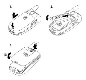
**Note:** Ensure that the battery cover is in place at the top and then clip into the bottom of the phone.
