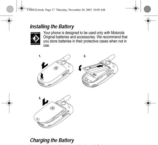
New batteries are shipped partially charged. Before you can use your phone, you need to install and charge the battery as described
