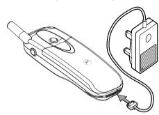
3 Insert the travel charger plug into a suitable mains power
