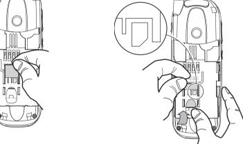
If the SIM card is inserted the wrong way round, or damaged, the Check Card message may be displayed. Remove the SIM card, check that it is the right way round and then re-insert it into the phone.
