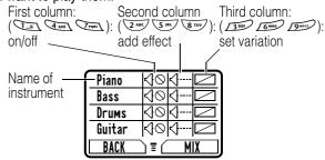
Press **MIX** ( $\square$ ) to play the mix file. Turn instruments on or off, add effects, and/or set an instrument variant using the following keypad keys.
