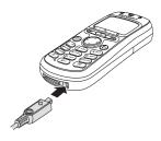
4 Insert the travel charger plug into a suitable mains power socket.
