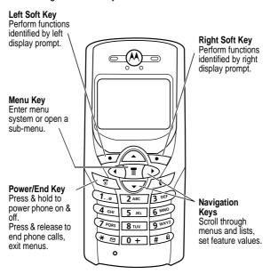
From the idle display, press To enter the main menu. Press to scroll through menu features in the main menu.
