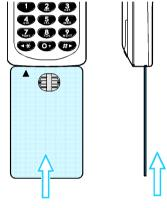
If the SIM card is inserted the wrong way round, or damaged, the Check Card message may be displayed. Remove the SIM card, check that it is the right way round and then re-insert it into the phone.
