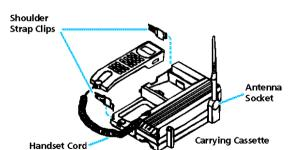
Attach the shoulder strap by sliding the clips into the slots in the carrying cassette. The clips will lock into place. To remove the shoulder strap, press the tabs and lift the clips.
